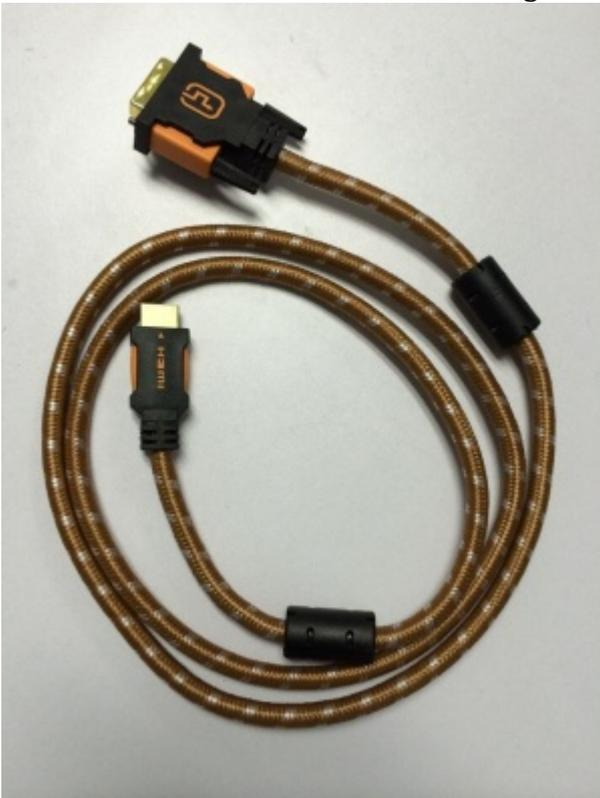
2. Connect the Orange Pi and the monitor using the HDMI cable as showed in the figure below.
